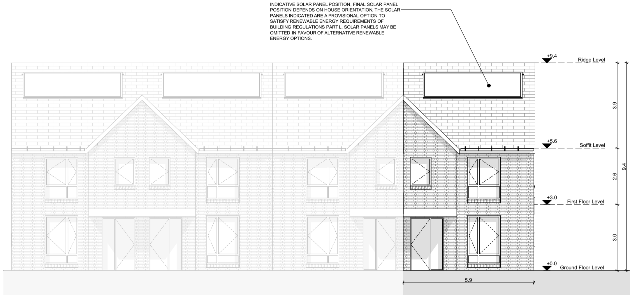
SCALE 1:100 Front Elevation
