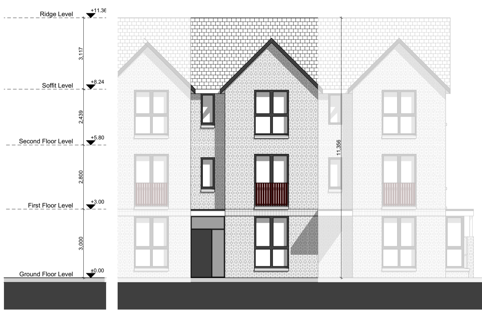
Front Elevation SCALE 1:100
