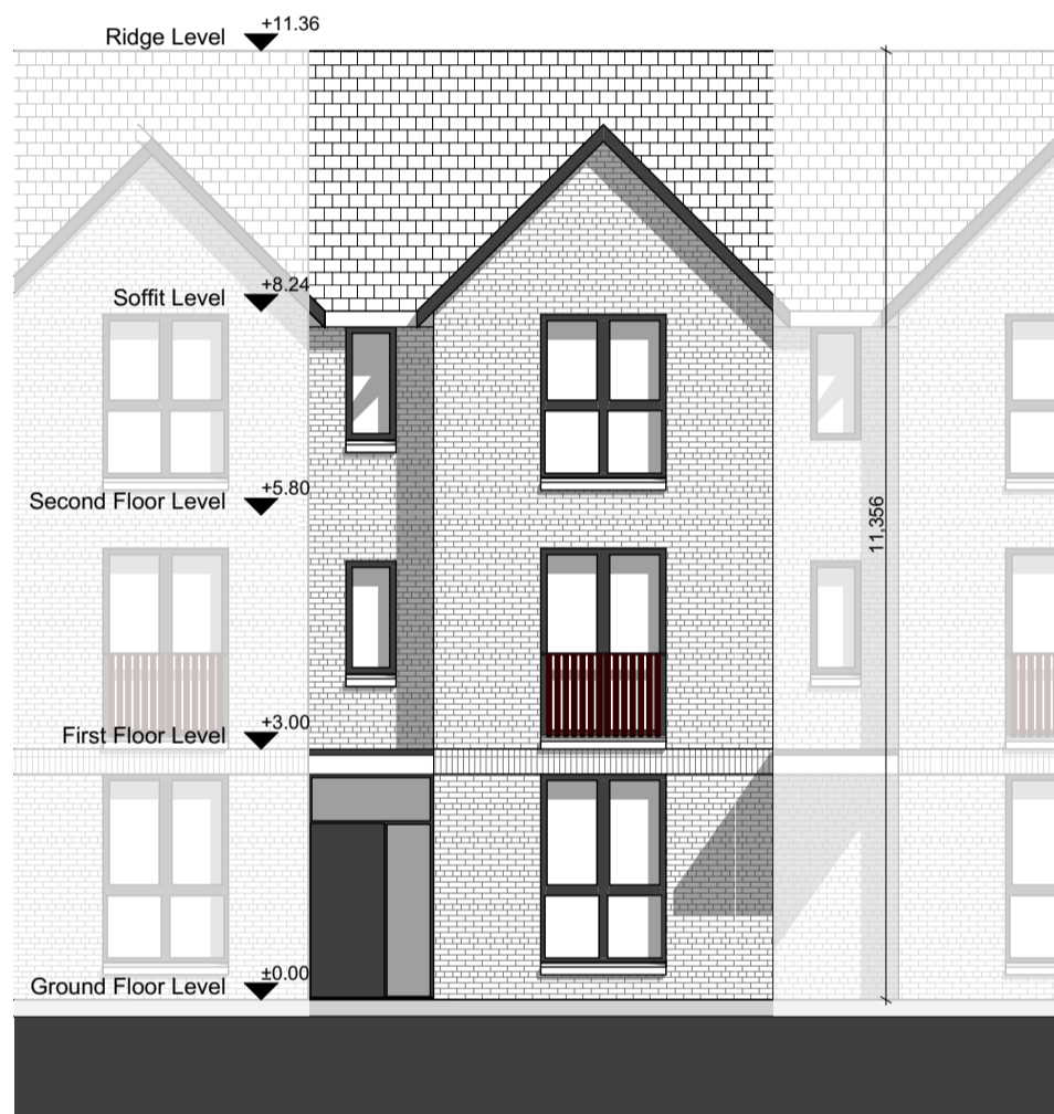
Front Elevation SCALE 1:100
