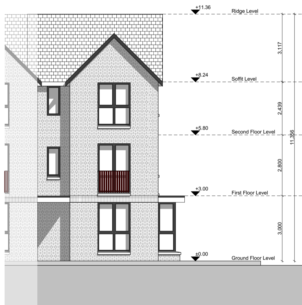
Front Elevation SCALE 1:100
