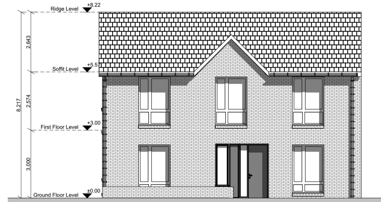
Front Elevation SCALE 1:100
