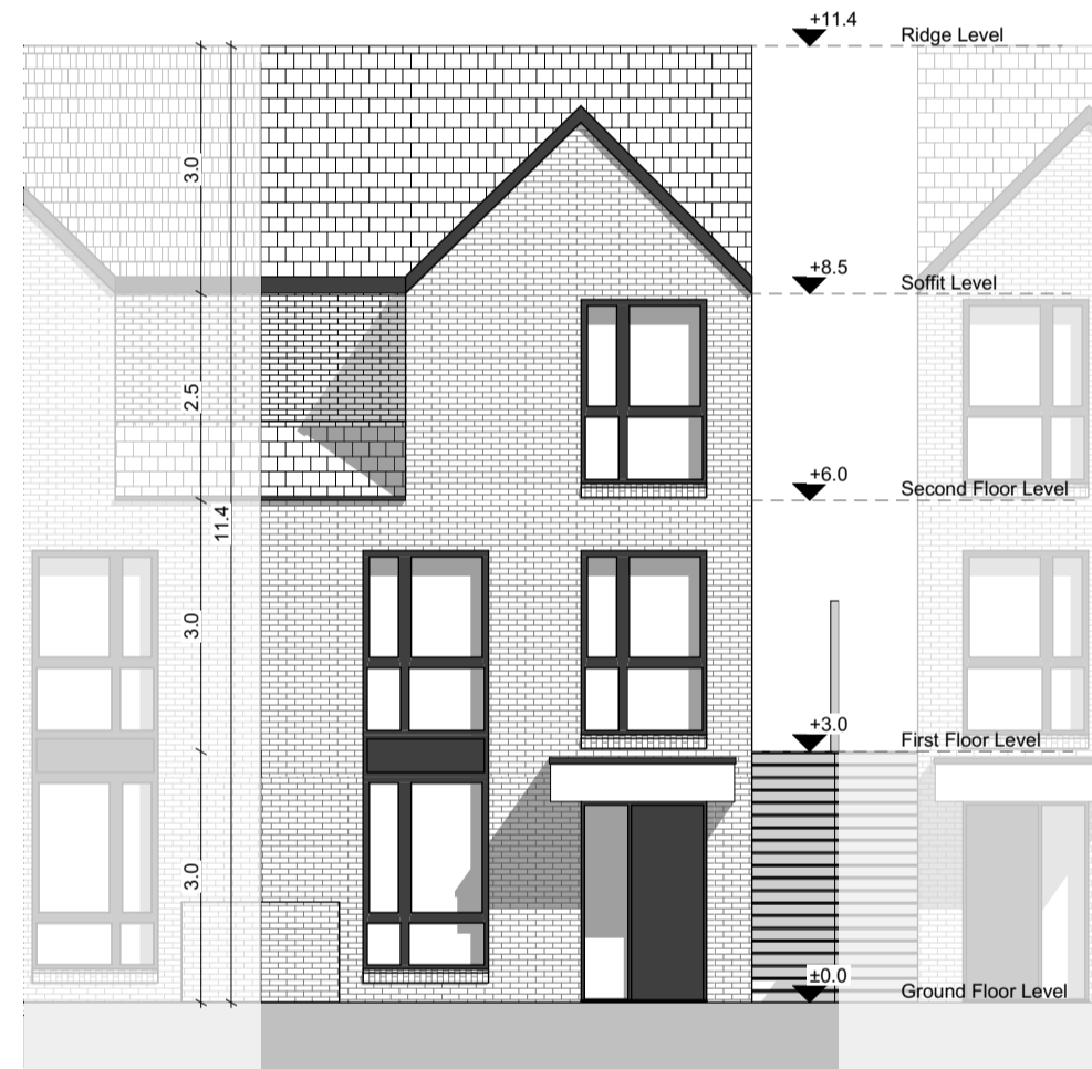
Front Elevation SCALE 1:100
